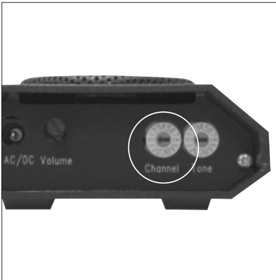
The personal code is selected using the tuner marked **Channel** on the back of CALL.
